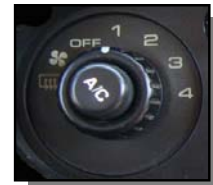
First Generation Mazda MX5 Miata Fan switch
